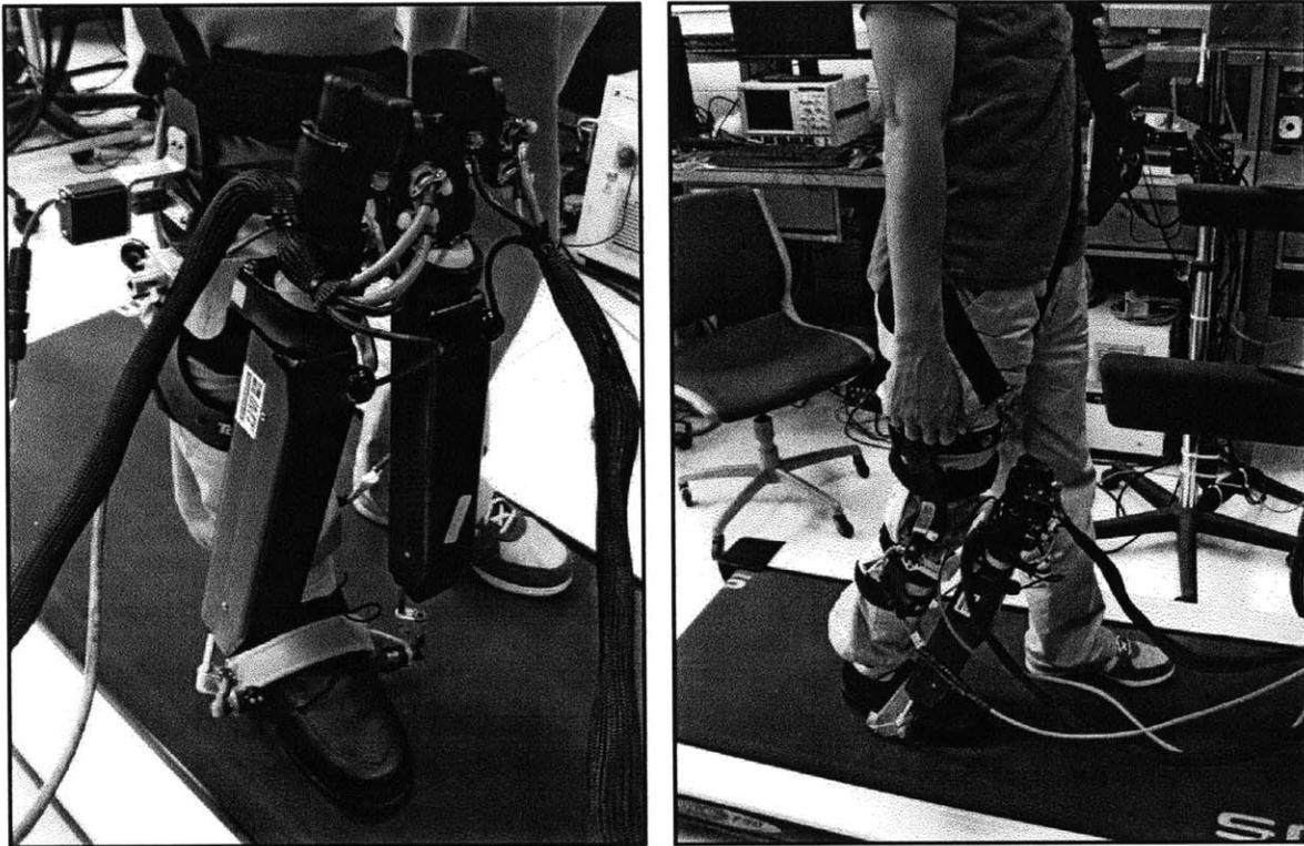
Figure 3.1 Experimental setup. Subject on treadmill wearing the Anklebot with custom shoe and knee brace.
