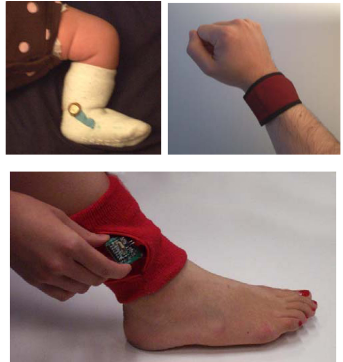
Fig. 4. Photograph of several form factors used: (upper left) baby sock with sewn electrodes, (upper right) wrist worn band, and (bottom) foot/ankle sensor band.
