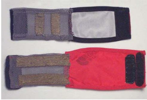
Fig. 5. Sample textile electrode configurations used for wrist sensor.
