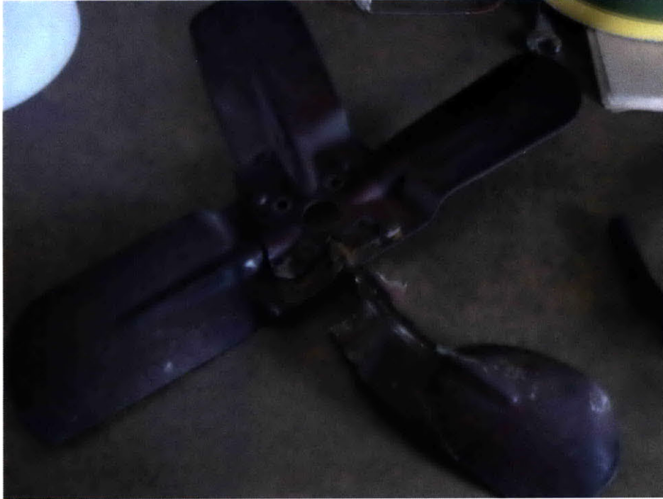
Figure 15: 1955 model fan that broke during testing.
