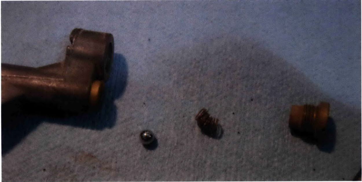
Figure 12: Exploded view of old power valve assembly. Notice spring failure.
