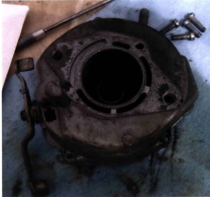
Figure 8: Bottom of carburetor before refurbishing. Notice gasket had stuck to the surface.
