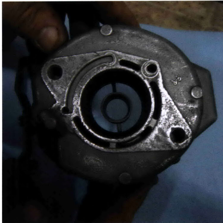
Figure 9: Bottom of carburetor after refurbishing. Old gasket removed, and surface cleaned.
