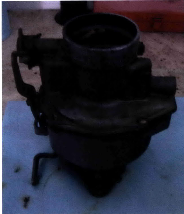
Figure 4: Carburetor removed from the engine before refurbishing. There is noticeable buildup on the surfaces of the carburetor.
