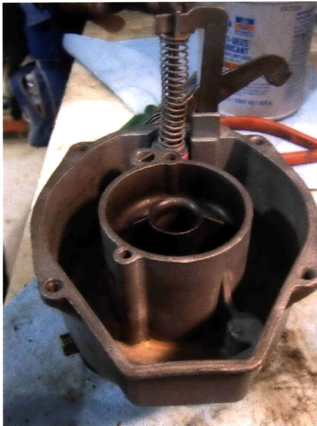
Figure 7: Carburetor bowl with sediment removed.
