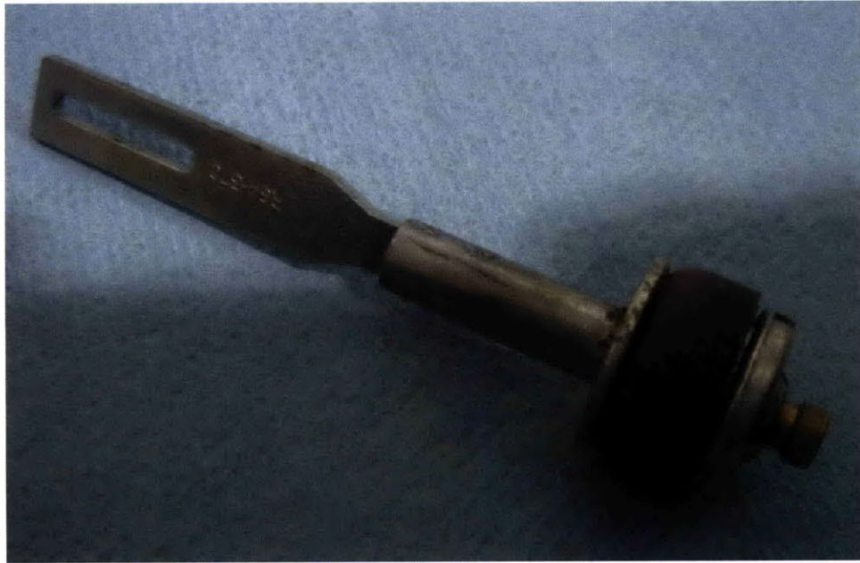
Figure 10: Old pump plunger with signs of wear.
