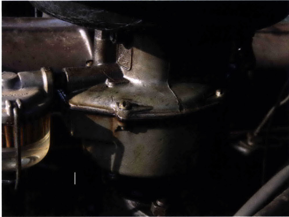
Figure 2: Carburetor installed on the engine before refurbishing. The outer surface had a shine that could have been caused by fuel leakage.
