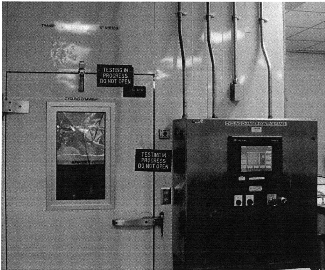
Figure 27: Vibration Table Cycling Chamber
