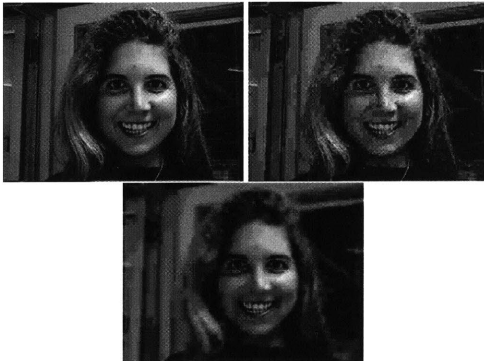
Figure 5-7: Preferential coding: the first image is the JPEG flat encoded image (File size of 14.1Kb); the second is a very low resolution JPEG encoded image using flat coding (File size of 7.1Kb); the third one is a preferential coding encoded image with high resolution JPEG for the eyes and mouth but very low resolution JPEG coding for the face and background (File size of 7.1Kb).
