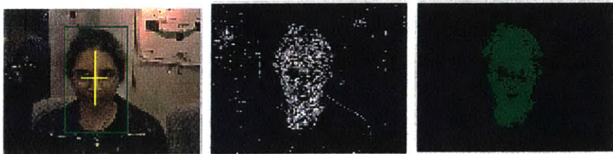
Face detection, per-pixel probability image computation and face blob growing
