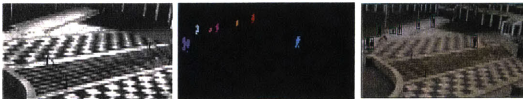
Background mean image, blob segmentation image and input image with blob bounding boxes
