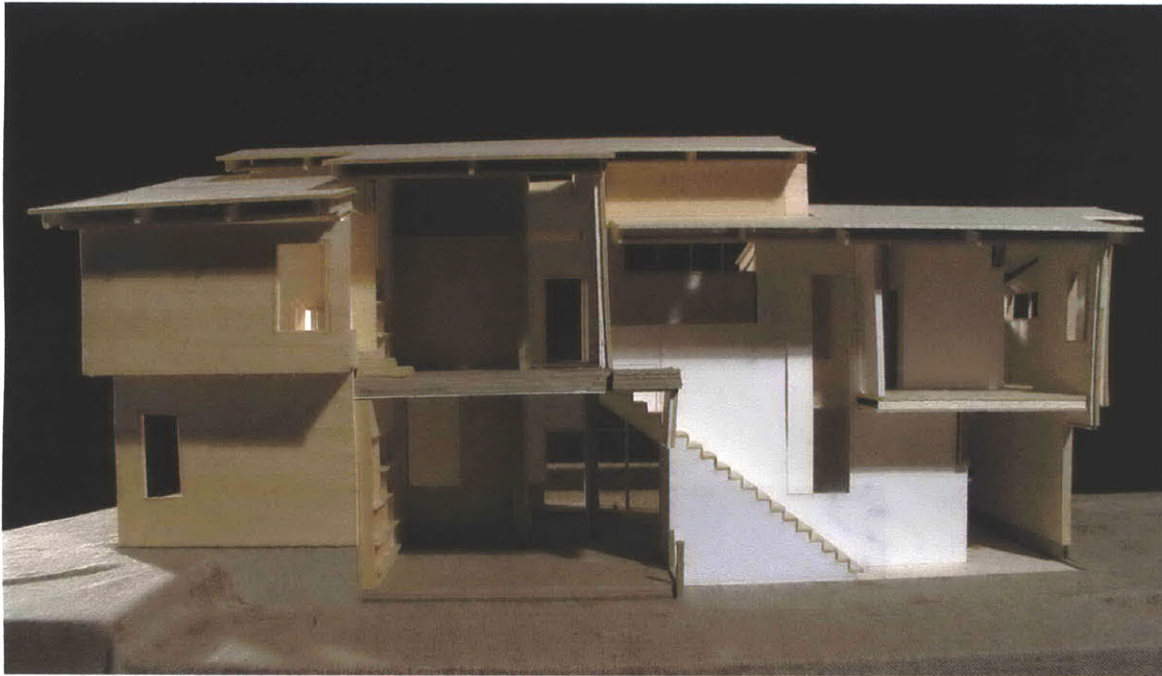
Sectional view of the building, from the north. In the center are kitchens for both apartments, and to the right is the second-floor's stair to its bedroom. The long rectangular window is translucent, providing light to the first-floor apartment's stair on the other side.
