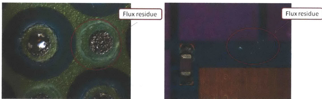
Fig. 3.1: Flux residue surrounding solder joints of BGA FET and on the board
