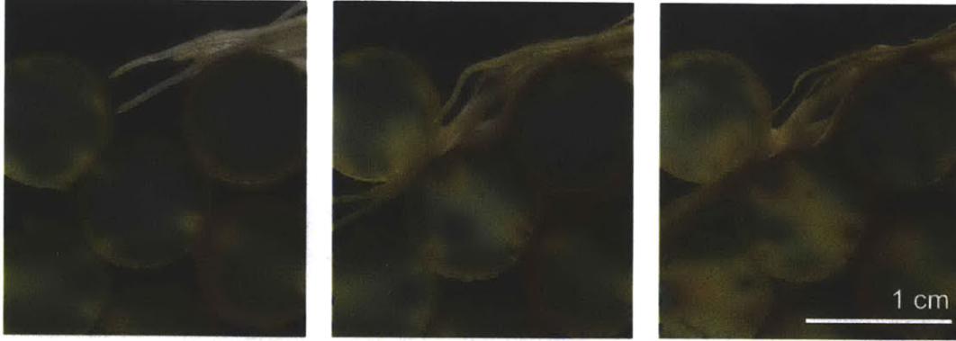
Figure 2-5: Roots exerting force into a granular system. Note that the center grain is subject to increasing stresses as the roots grow around it. Time between images is approximately 20 hours.
