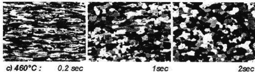
Figure 6: Annealing treatment of cold rolled aluminum demonstrating grain growth [13].
