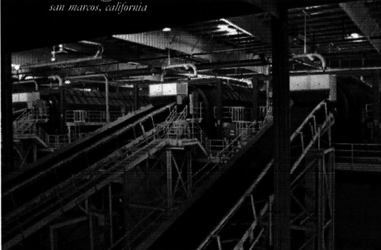
series of conveyor belts leading to trommel screen machines
