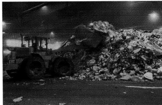
front-end loader moving trash at a conventional transfer station's tipping floor
