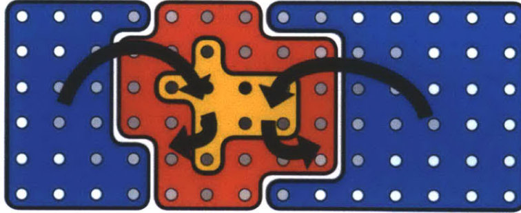
Figure 29. Overflow of net sink areas as inventories deplete. Additional vehicle flow from net sources to net sinks is pushed outwards. As a result the area of net sinks increases while the area of net sources decreases (red area)
