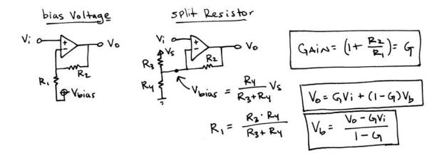
$$\frac{V_{i}-V_{b}}{R_{i}} = \frac{V_{b}-V_{i}}{R_{2}} \rightarrow V_{b} = \frac{R_{2}}{R_{i}}(v_{i}-V_{b})+V_{i}$$
