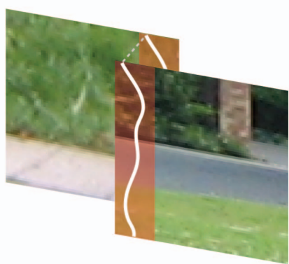
Fig. 2. Illustration of how we compute the left-right seam energy for two overlapping patches. The white line is the seam along which the color difference between the patches is minimum. The color difference along the white line is defined as the seam energy.
