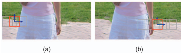
Fig. 17. A local jittering scheme can fix some types of misalignments, but has limitations, motivating the use of an MRF to jitter patches globally. (a) The misalignment between the red patch and the patch to its right can be reduced by jittering the red patch toward the right. (b) A simple local jitter operation cannot fix the misalignment error for this example. Moving the red patch upward would better fit the side on the right, but it would cause misalignment with a patch on its left.
