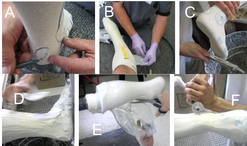
Figure 1 Traditional fabrication process of an ankle foot orthosis for a patient.
