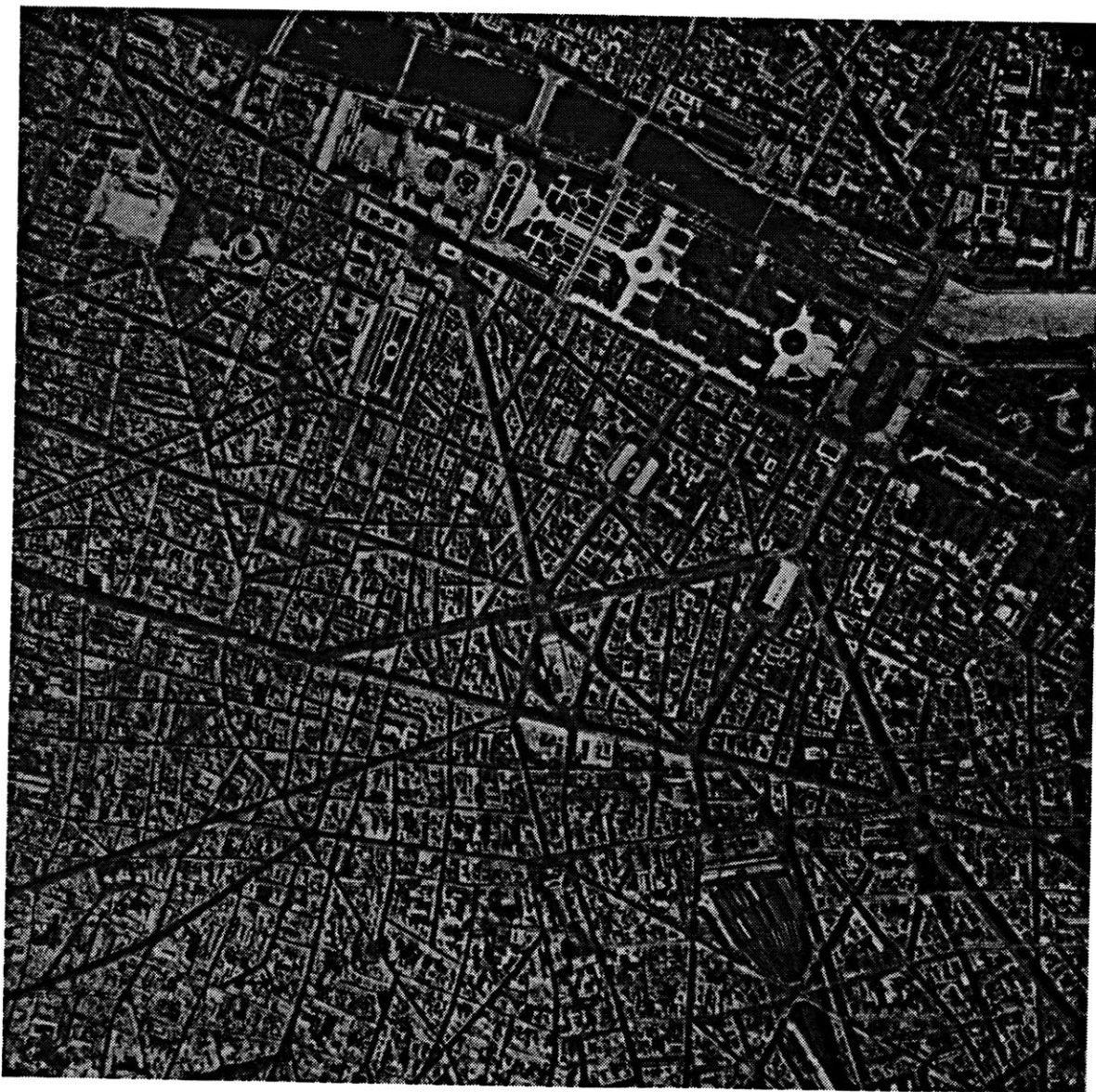
Figure 62: Haussmann's design for Paris. Notice nodal network of wide streets superimposed upon the pre-industrial city fabric. Haussmann's design for Paris influenced Robert Napier's plan for the social and political control of Lucknow.
