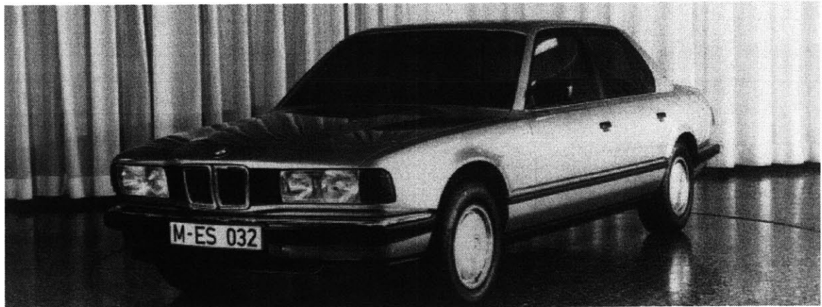
Figure 2-34: Another final picture model of a proposed BMW 7-Series. Reproduced from [Wic87].
