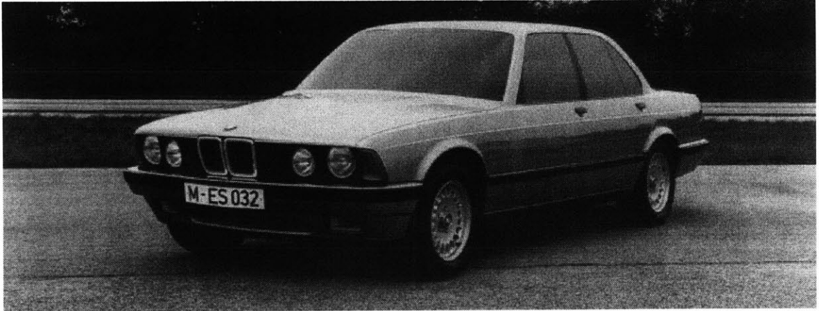
Figure 2-33: A final picture model of a proposed BMW 7-Series. Reproduced from [Wic87].
