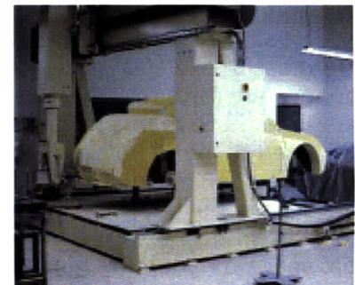
[1.9] C-tek's CNC 5-axis milling machine produces full-scale car models.
