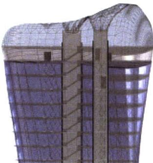
[7.1] This section shows the expansion of floor slabs on the top of the composite tower.
