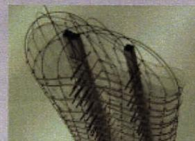
This model further represents the form of the tower, using plastic and metal wires. Because of the material property of the composite strips, they will have to be continuous at the top of the tower in order to eliminate any stress concentrations at connections. Holes at precise locations are cut from the plastic floor plates using the laser cutter, and stainless steel wires are fed over the top and through these holes to illustrate the "head" form of the tower.
