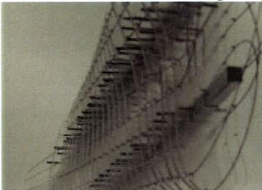
This model further represents the form of the tower using plastic and metal wires. Because of the material property of the composite strips, it is important that they are continuous at the top of the tower in order to eliminate any stress concentrations at connections. Holes at precise locations (drawn in CAD) are cut from the plastic floor plates using the lasercutter, and stainless steel wires are fed through these holes and over the top to illustrate the "head" form of the tower.
