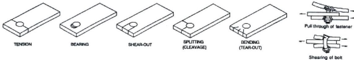
[4.7] various modes of failure of bolted connections in polymer composites
