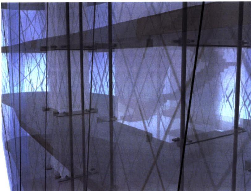
[5.92] This perspective shows the interior component at the core of the tower. While each floor slab is supported by a set of composite cables that goes around the interior up to the cores, a number of roller/damping joints are fastened at the connection between the core and hole of the floor slab to allow for some flexibility.
