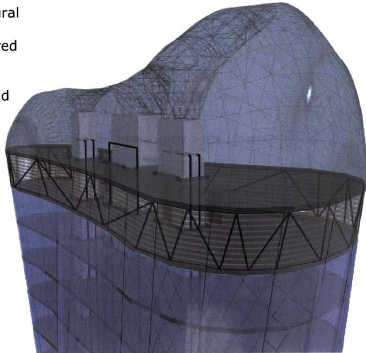
[5.91] This closeup view of the top of tower shows structural assembly of the steel cage "cap", mushroom columns, transverse slabs, three concrete cores, and supporting cables.
