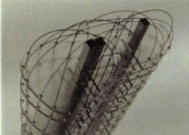
**tower structure model: plexiglas, brass tubes, stainless steel wires**
