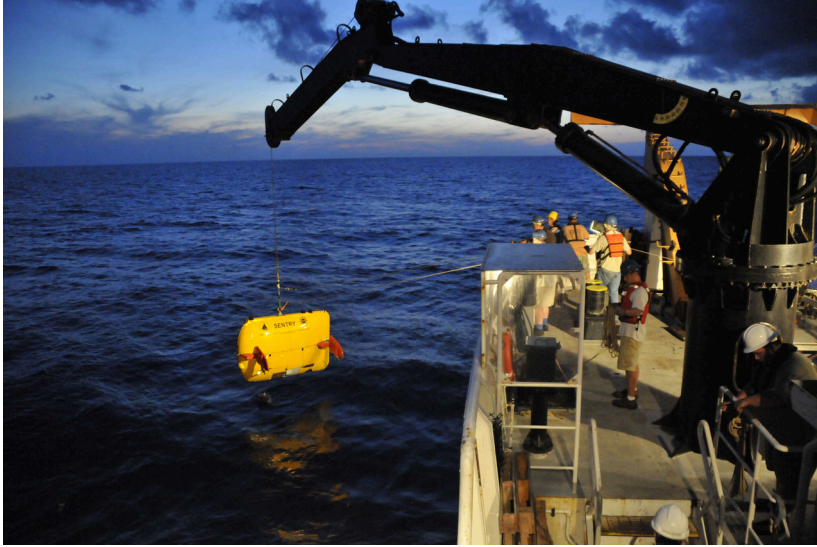
Figure 1-20: The NDSF AUV Sentry is an unmanned oceanographic research vehicle that dives as deep as 6500 meters to perform various scientific missions. Sentry navigates primarily by DR with a FOG and DVL. The FOG is located in the main pressure housing, roughly amidships and just below the name label. The DVL is on the keel just aft from the bow. The large separation between these sensors on a vehicle that may deform under extreme pressure (even slightly), motivates our study of stable, in-situ sensor alignment methods. (photo credit: D Yoerger, ABE/ Sentry Group, WHOI)
