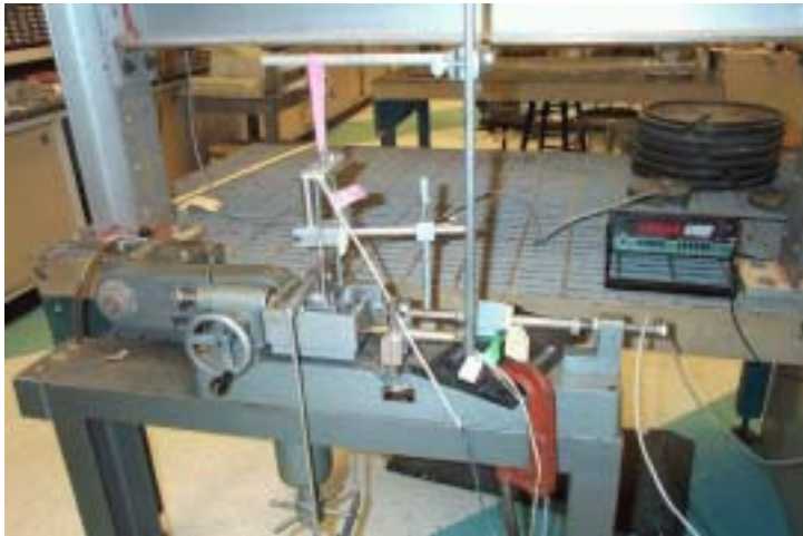
Figure 6.11: Direct shear box and test assembly used for measuring the soil internal friction angle. This system has been modified so that the mass of the upper half of the shear box can be suspended from above. This allows us to test with much lower normal loads.
