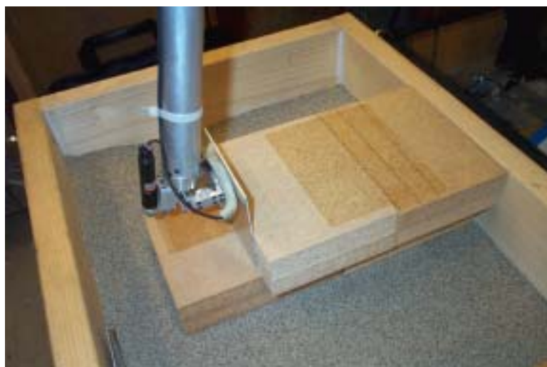
Figure A.2: In order to estimate arm flexion, the end of the arm is immobilized while the motors drive the arm into the obstruction.
