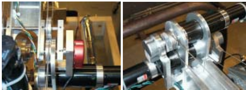
Figure A.1: External encoders for the shoulder and elbow motors. The shoulder encoder is mounted directly on the joint, whereas the elbow encoders are at the motor output shafts.
