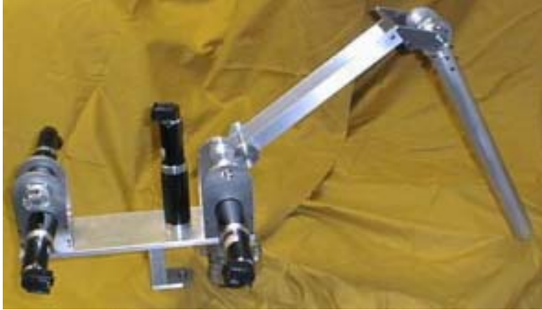
Figure 3.1: The original manipulator design, un-cabled, before the modifications and additions to make it fully functional. Rotary compliant elements were to be placed in the base and shoulder and linear compliant elements were to be placed in-line with the cabling in the open space above the horizontal base platform.
