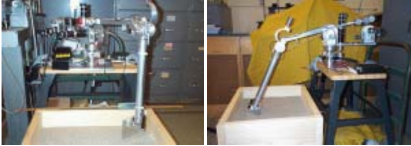
Figure 5.2: Front and side view of the manipulator arm executing and completing a digging sequence in the sandbox. The origin of the manipulator coordinate frame is located directly below the shoulder joint at the level of the table surface. The soil surface is typically located at z = -13'' in the manipulator frame. Insertion forces are primarily generated by the shoulder joint, and stroking forces are primarily generated by the elbow joint.
