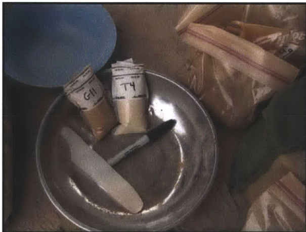
Figure 3-10: Sub-samples collected for particle size analysis
