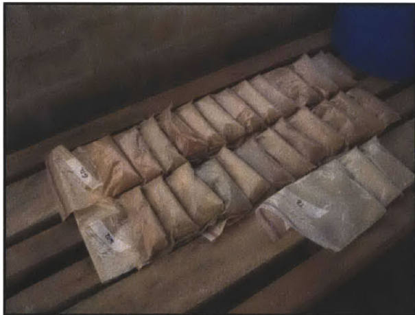
Figure 3-9: Sub-samples of pounded, sieved clay for soil tests
