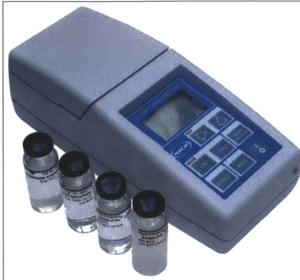
Figure 5-1: Hach 2100P turbidimeter (Filtration Technology Ltd.)
