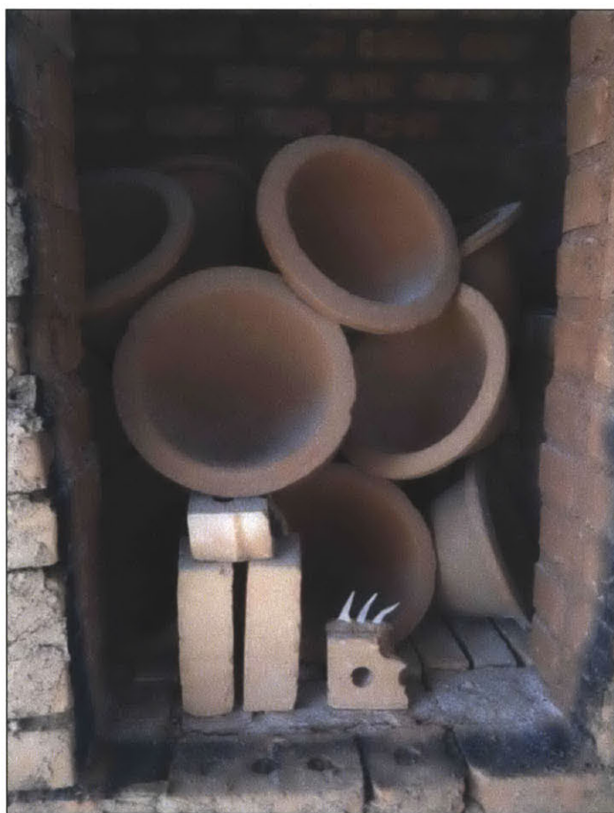
Figure 4-15: Filters stacked in kiln (Manny Hernandez)
