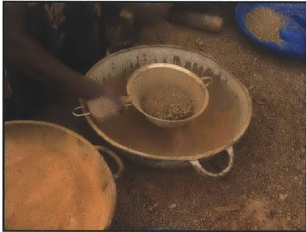
Figure 3-8: Sieving the clay to remove gravel
