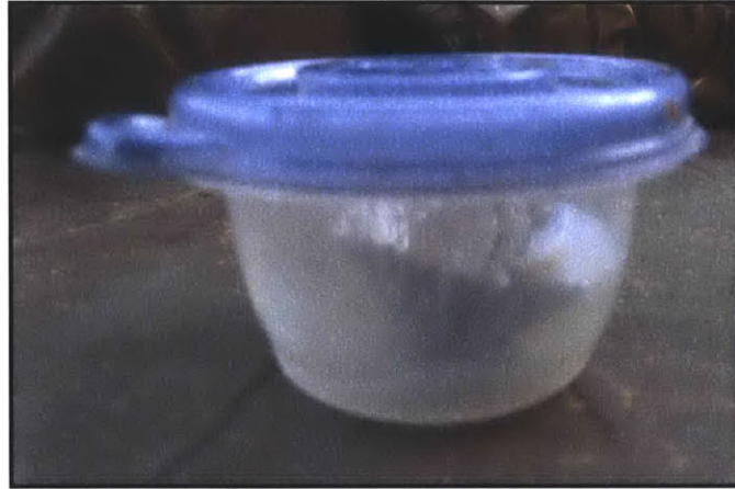
Figure 3-20: Sample placed in Tupperware® to maintain water content
