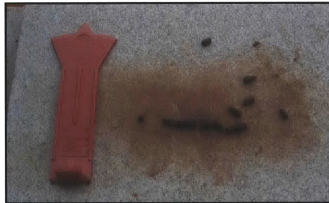
Figure 3-19: Clay thread crumbling at 1/8 in.
