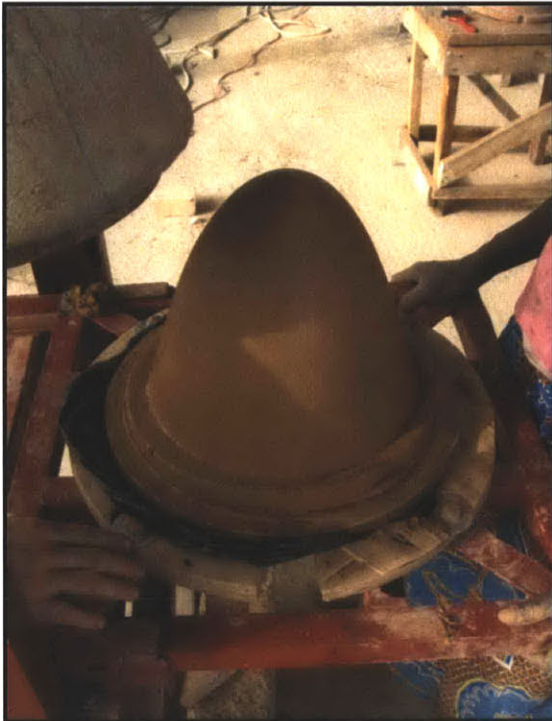
Figure 4-13: Inspecting the pressed filter
