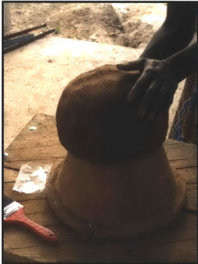
Figure 4-5: Pre-forming the filter
