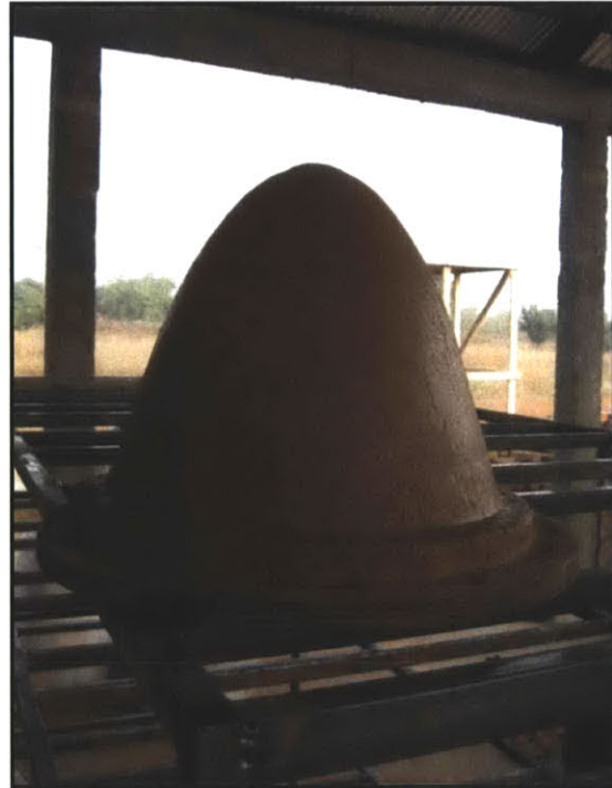
Figure 4-14: A finished filter on the drying rack
