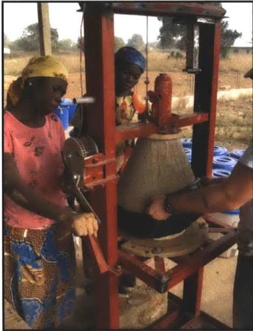
Figure 4-7: Lowering the female mold
