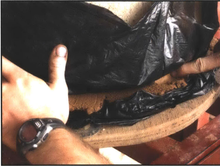
Figure 4-11: Clay squeezing out from between the molds
