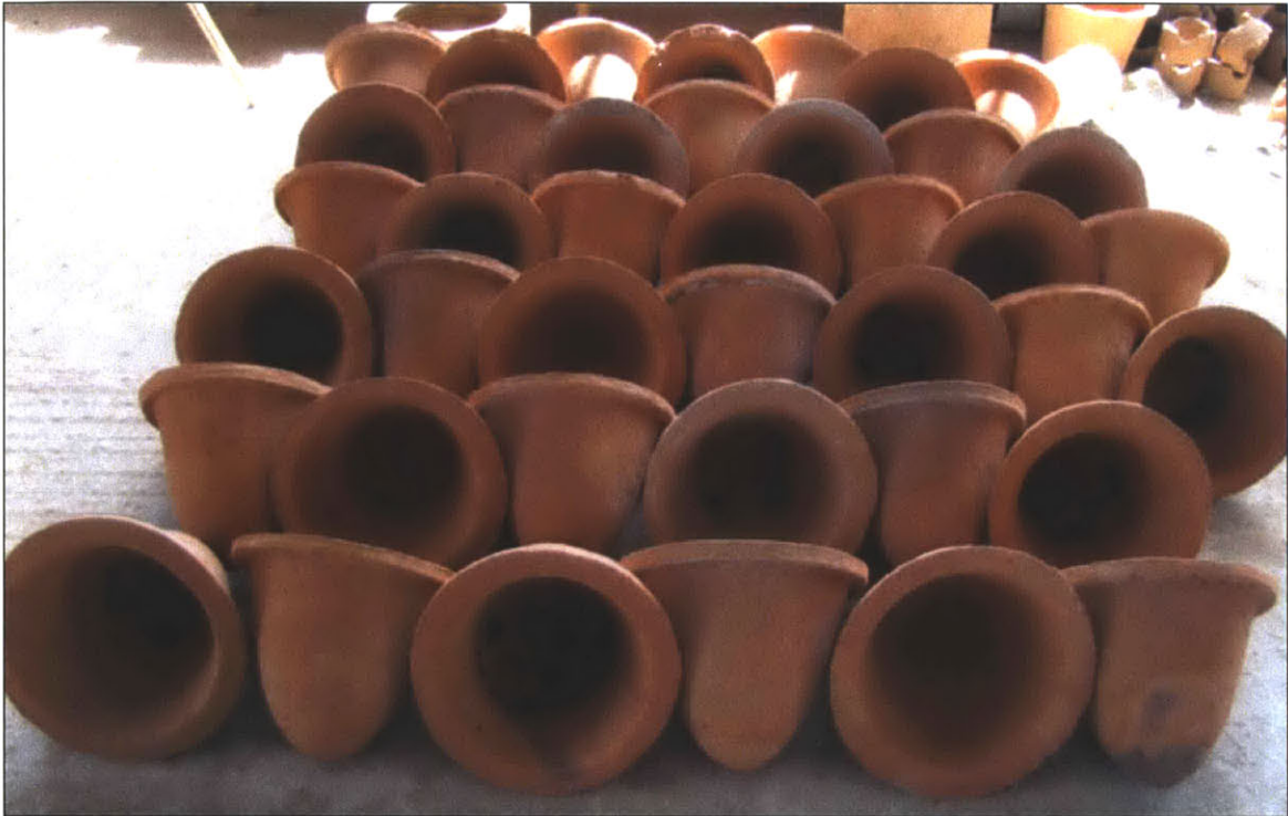
Figure 7-3: Incomplete firing using first spacer revision
