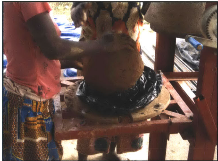
Figure 4-6: Forming the clay on the male mold
