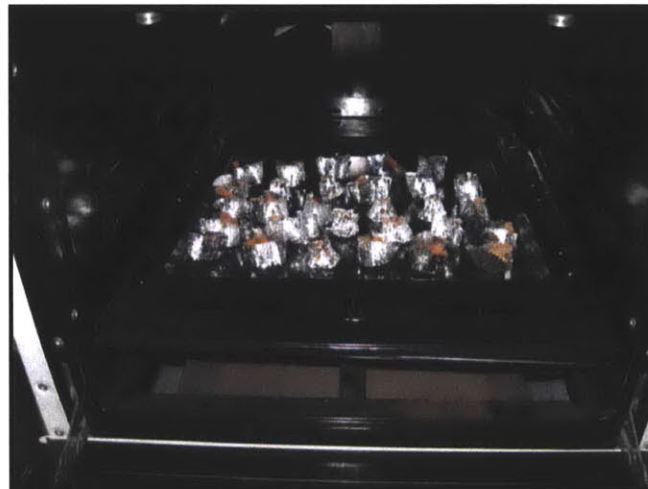
Figure 3-17: Sub-samples drying in oven
