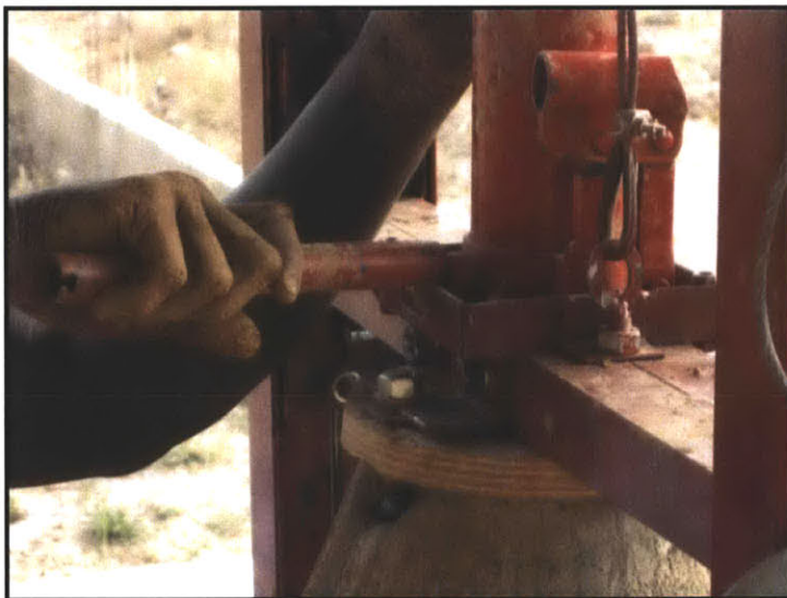
Figure 4-9: Affixing the lever to the jack
