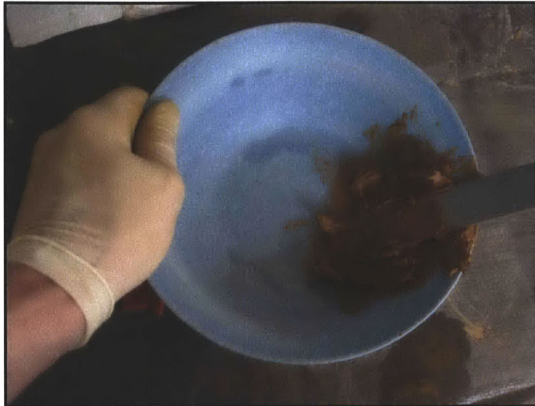
Figure 3-11: Mixing clay to adjust water content
