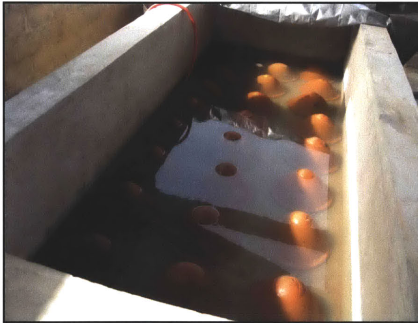
Figure 5-2: Fired filters soaking in saturation tank
