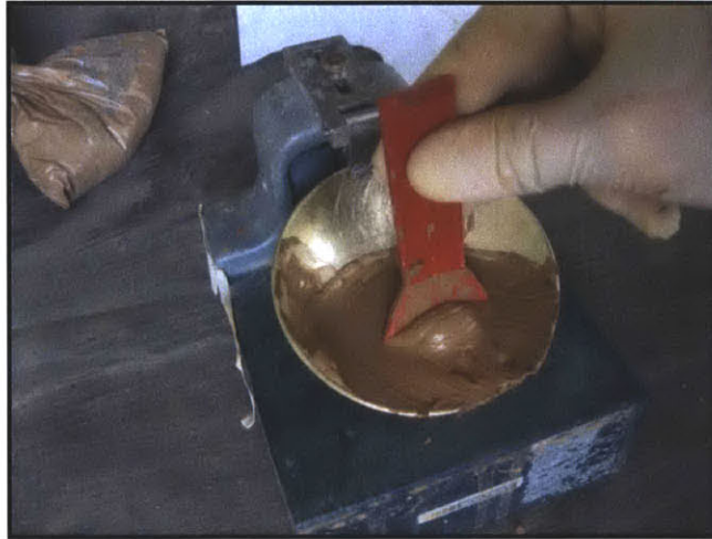
Figure 3-13: Grooving the pat of soil
