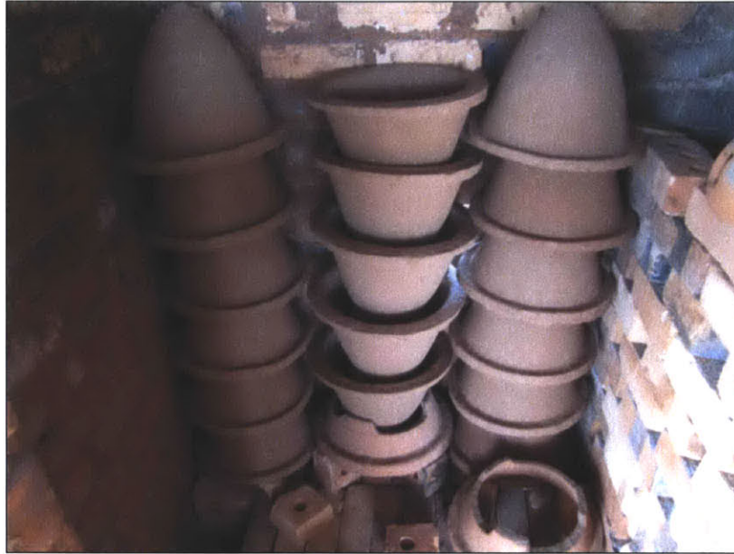
Figure 7-1: Filters stacked in kiln with first revised spacer
