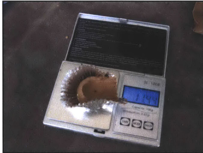
Figure 3-16: Weighing the sub-sample on a digital scale
