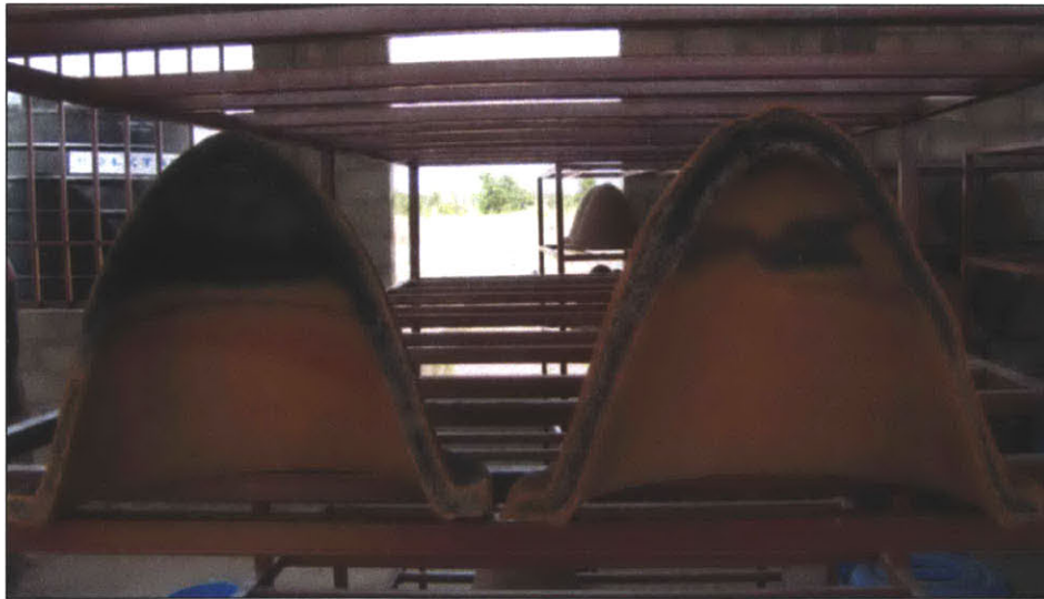
Figure 7-4: Incomplete firing (cross section)
