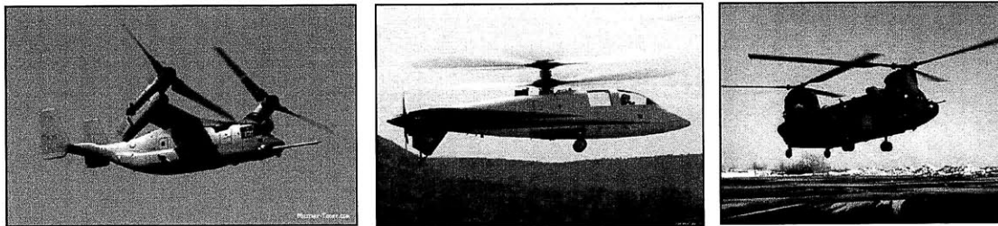
Figure 2: Rotor Systems - Tilt /Coaxial /Tandem (Military Today/Flight Global/Airliners)
