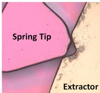
Fig. 3. DRIE spring tip of the ionizer main body substrate locked into a notch on the boundary of the extractor substrate. The main body substrate has eight springs that are evenly distributed across the boundary of the extractor to assemble the extractor substrate to the rest of the ionizer.
