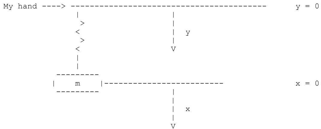
$y$  is the position of the plunger, relative some choice of zero point. Arrange it so that if  $y = x = 0$ , the mass is at rest. A constant upward force on the mass exerted by the spring cancels gravity, and we simply ignore both. The "relaxed" position of the rubber band just cancels the force of gravity.
