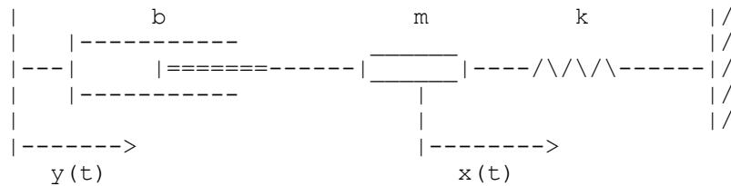
We are driving the system by motion of the far end of the dashpot, while keeping the far end of the spring constant.
