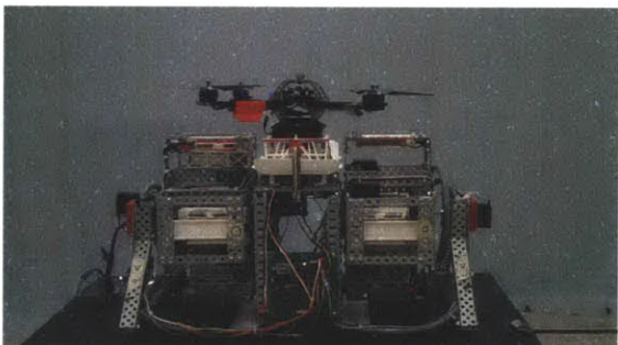
(f) After the battery swap is finished, the clamps (right to left) are released
