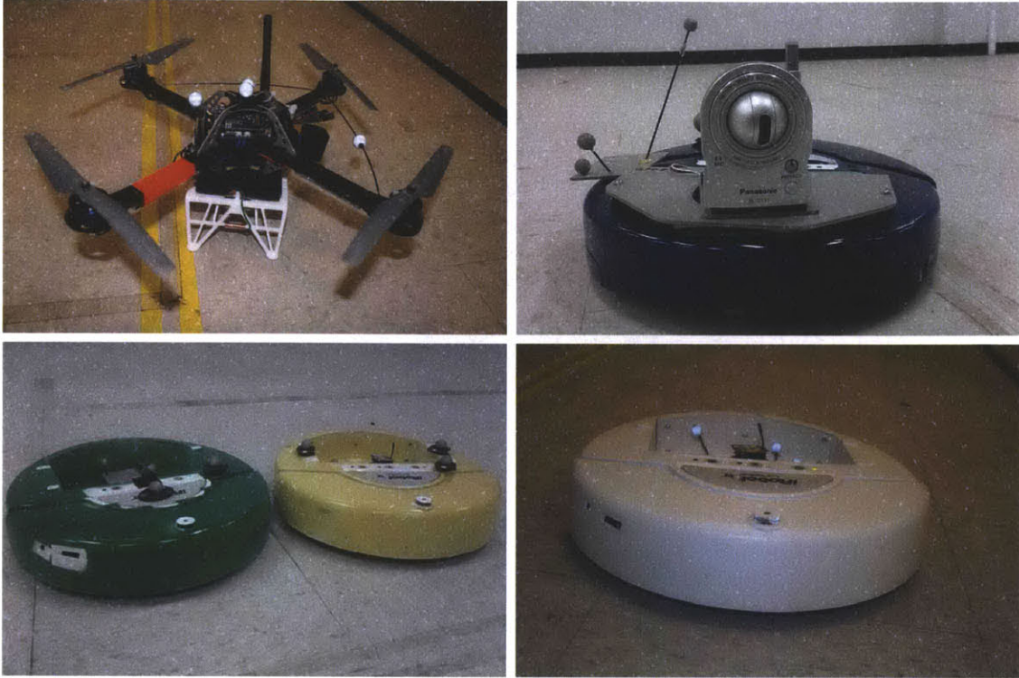
Figure 6-8: Four agent platforms used in flight experiments: Team UAV (top left), Team UGV (top right), Target UGV (bottom left), and a Civilian UGV (bottom right).
