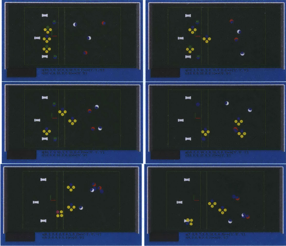
Figure 6-2: A simulated persistent surveillance mission (PSM) using the centralized multi-agent MDP (MMDP) formulation. The agents must coordinate to ensure no gaps in surveillance coverage while maintaining a communication relay.
