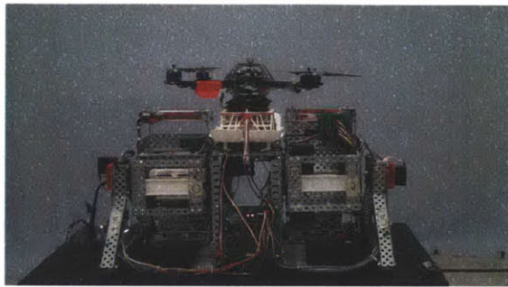
(b) Quadrotor clamped to pad with shore power land
