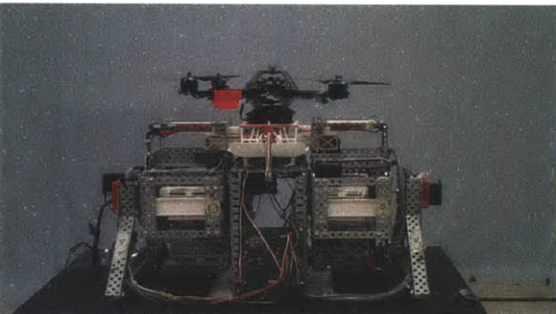
(e) Replacement battery pushed into place (right to left), moving the old battery into the left drum
