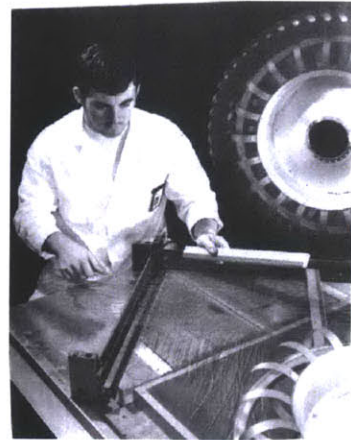
Figure 3 - A worker hand weaves wire for LRV wheel (Image Courtesy of NASA)
