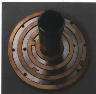
Figure 24 - Copper electric slip rings mounted to outside of inner hubcap
