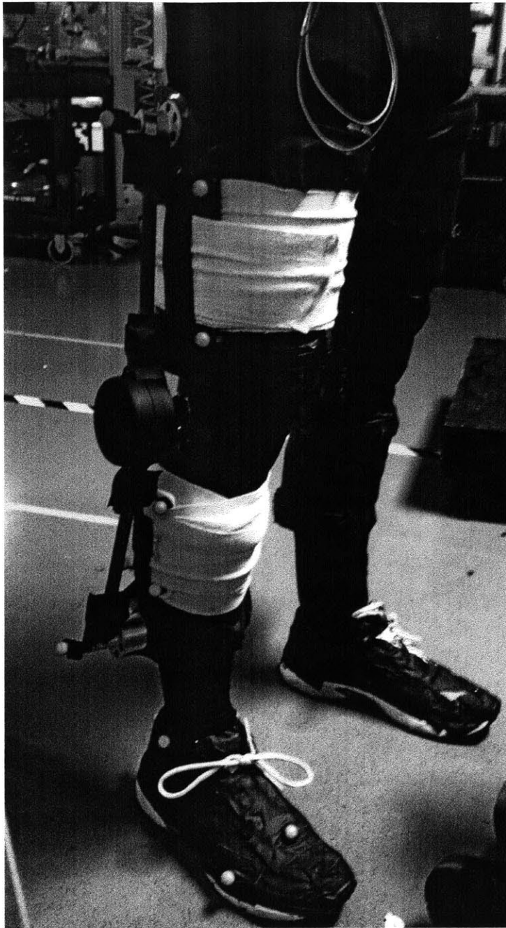
Figure 5-1: Right leg instrumented for motion capture. Black tape covers all reflective surfaces.
