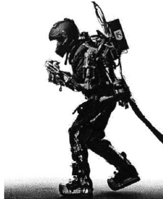
(b) Active Sarcos exoskeleton, hydraulic with an offboard compressor (not shown) [40]
