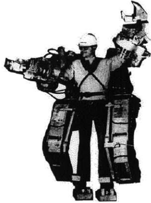
(a) Active hydraulic driven Hardiman, the legs of which were never used [35]
