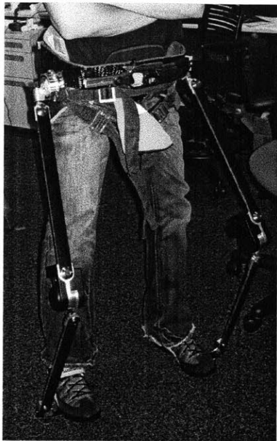
(a) Pelvic harness with toe attachment
