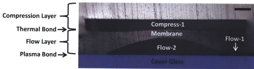
Figure B-6: Cross-section of the microfluidic device showing the immobilization region. The device is vertically cut along the line from port-B to port-C . The thermally bonded compression layer and flow layer are visible. The PDMS channel array is molded from the flow-1 layer with 10 \mu\text{m} thickness. A 15-20 \mu\text{m} thin PDMS membrane is formed between the compress-1 and flow-2 layers. This device would later be plasma bonded to a cover glass. The fabrication tolerances are listed in Table B.1. Scale bar: 50 \mu\text{m} .
