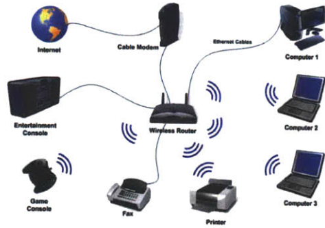
(a) An example of modern home network : various devices and applications share the same wireless channel from a single access point
