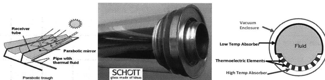
**Figure 5-1: (left) Cartoon of a solar parabolic trough collector array. (middle) Photograph of a receiver tube. (right) Schematic, cross sectional view of the proposed receiver tube of the solar thermoelectric topping cycle.<sup>69</sup>**
