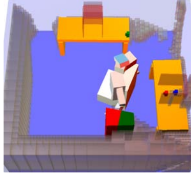
(b) The sub-regions are too big; the closer sub-region is split again.
