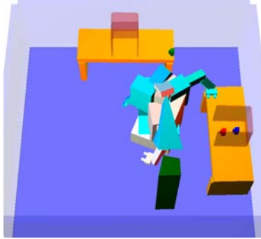
(d) A look pose (cyan) for the robot to stand so as to look at the target region (green) is generated.
