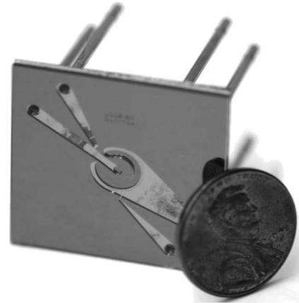
Fig. 9. Optical image showing an assembled turbopump device.
