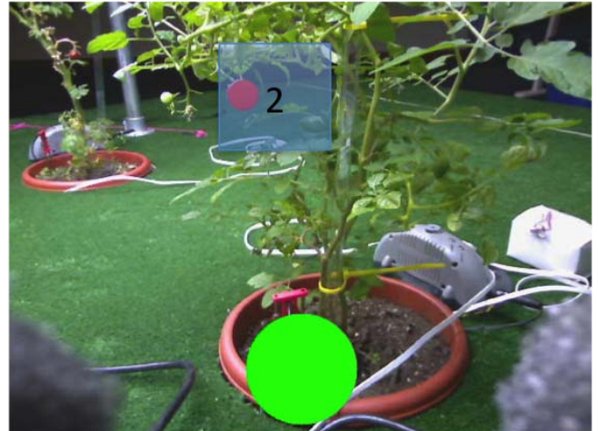
Fig. 11 Image-based visual servoing: actual fruit location within inventory location 2 (red dot) and desired fruit location within the gripper (green disc).
