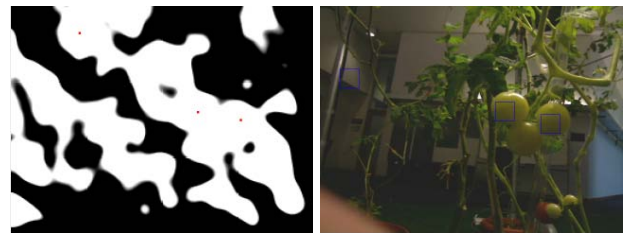
Fig. 7 Left : Result of convolution of input image with 40 feature/location pairs. Red dots correspond to local maxima. Right column : Detected fruits are highlighted with a rectangle. Notice the false-positive and misses in the bottom row.
