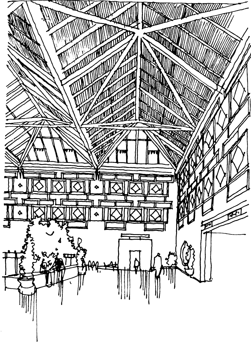
Fig. 2.8 The lobby of Fragrant Hill Hotel The 105 ft by 110 ft atrium is enclosed by steel space frames.
