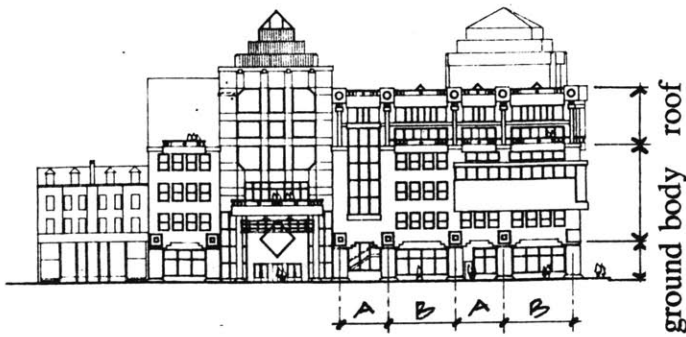
Fig. 5.25 Facade composition The width, the height and the width of the window the Hayden Building become the new building facade composition rules.
