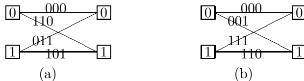
Figure 20: Trellis sections of (a) rate-1/3 2-state binary convolutional code \mathcal{C}_1 ; (b) similar code \mathcal{C}_2 .
