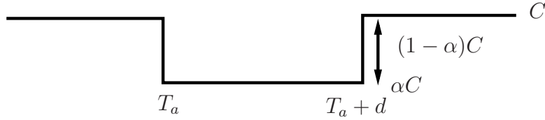
Figure 4-4: Depiction of the capacity profile under a weather-front based uncertainty set for a single affected airspace element. The plot is for a particular realization of the parameters (T_a, d, \alpha) .
