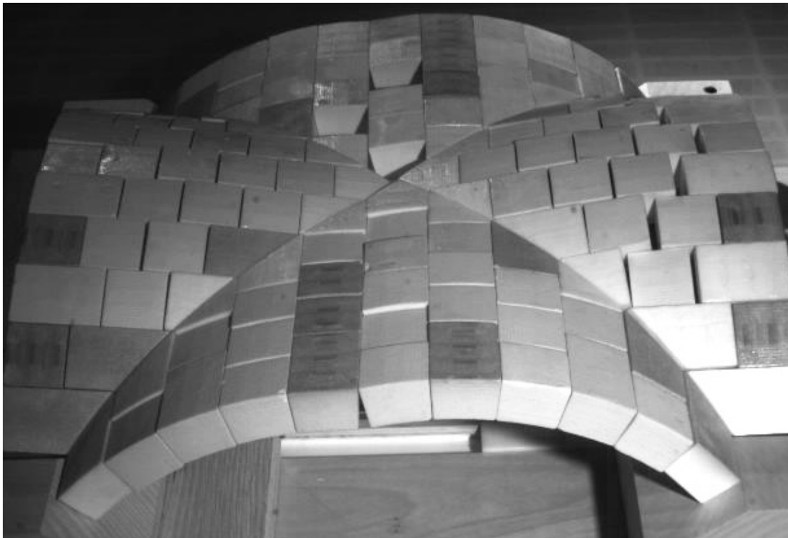
Figure 3.2: The groin vault cracks along the crown of the vault and the perpendicular arms crack linearly. A few blocks fall out at the crown, indicating that they do not carry any compression forces.
