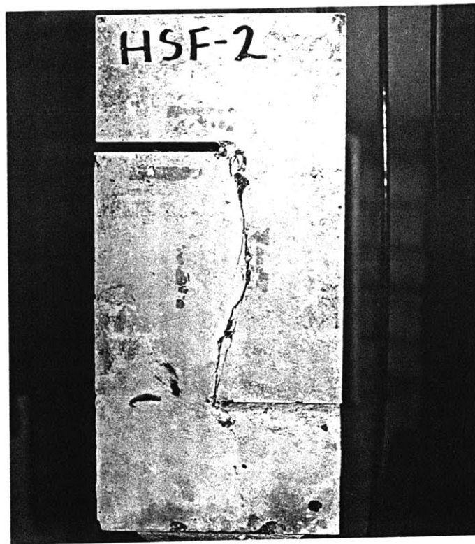
Fig. 5.15 SHC specimen after failure.
