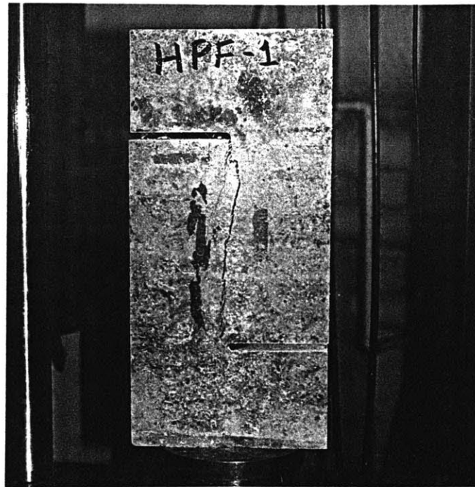
Fig. 5.13 PHC specimen after failure.
