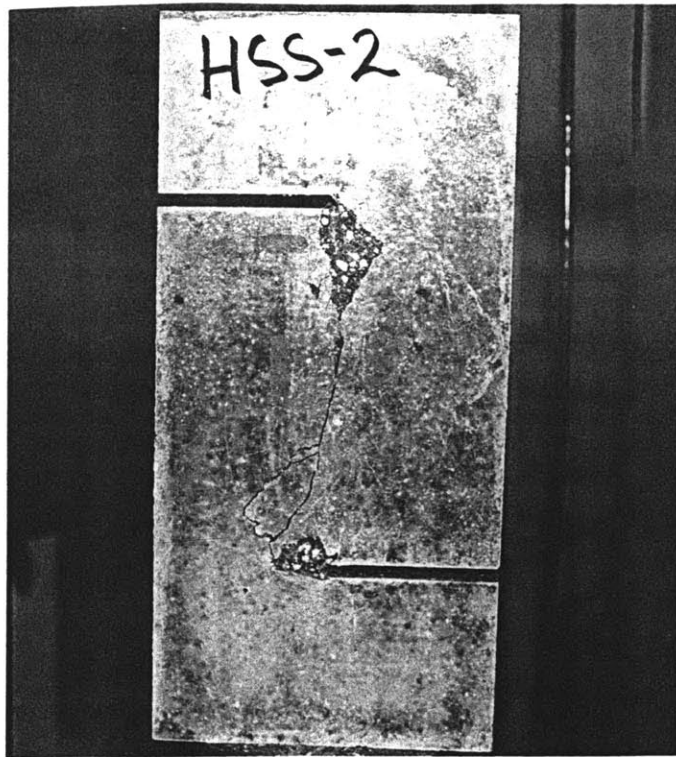
Fig. 5.17 HCS specimen after failure.
