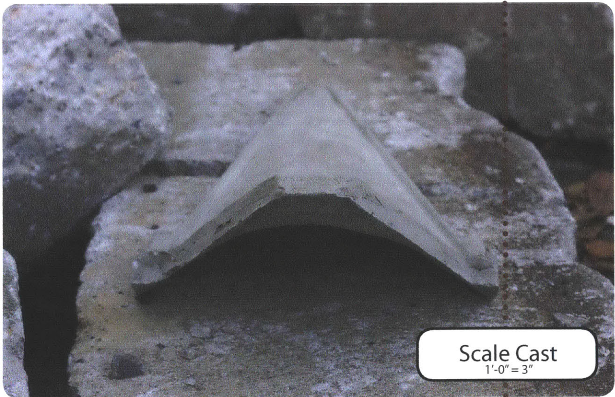
Dec 3rd | Photo of typical wall module (saddle shape) cast
