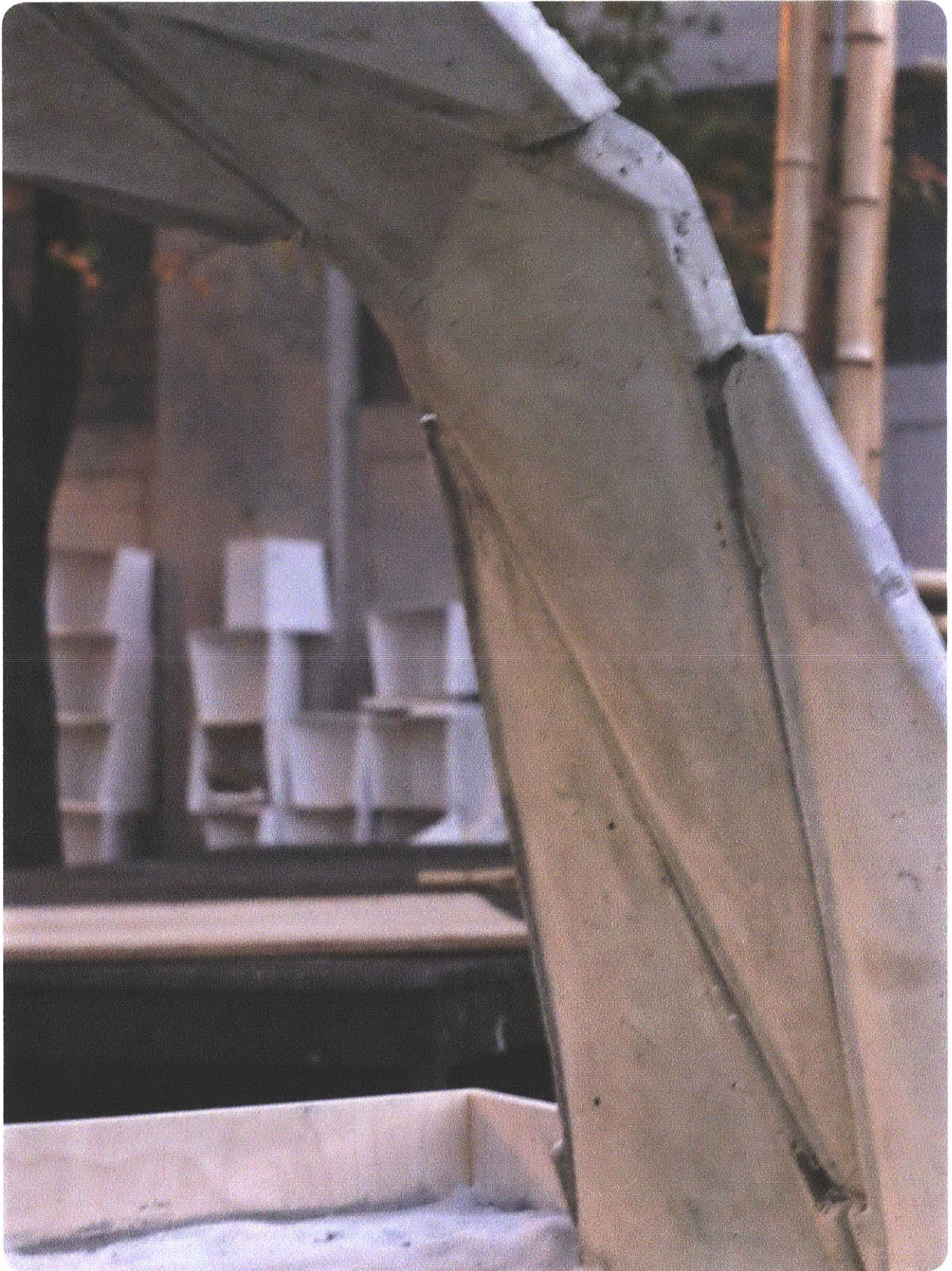
Photo of molded surface finish from within the scaled assembly
