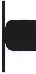
Figure 6: Outline of a flag with a saturating exponential H(x) profile. For such a flag, D^*H(0) \ll D^*H(x>0) and the oscillation should resemble that of a rigid plate pivoted at x = 0 .
