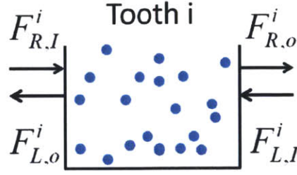
Figure 2-2: Diagram of incoming and outgoing, left-going and right-going fluxes for a single tooth, i , of the system.
