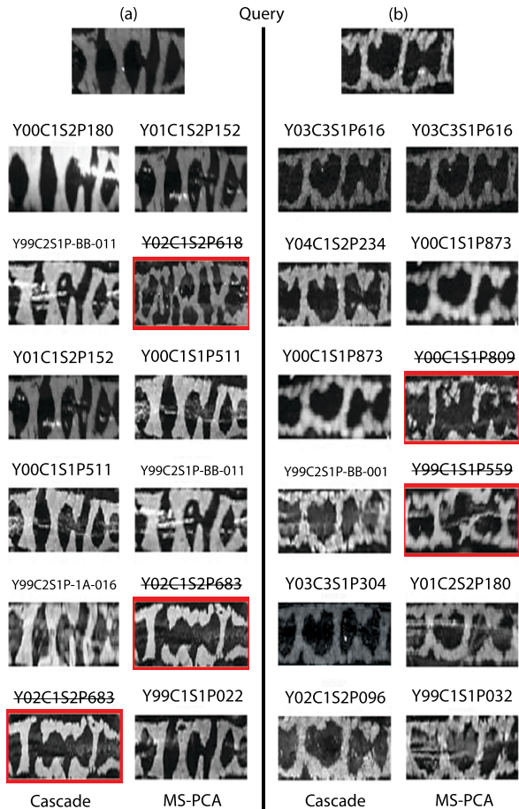
Figure 8. Two sample retrievals comparing the deformation invariant matcher and MS-PCA. The queries are marked (a) and (b) and the retrievals proceed in rank order down a column per method (self-matches are omitted and appear at rank 1). Mismatches are highlighted in red and their labels are crossed out.
