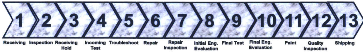
Figure 9: Ideal Repair Process
