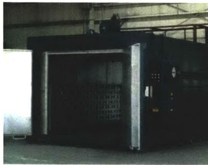
Figure 19: Walk –in vacuum-bake chamber, five of which are located in the pilot area
