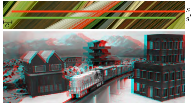
Figure 4: A 2D EPI of a light field, showing two planar u - v -cuts. The horizontal offset c changes the convergence plane of the stereoscopic image pair. The bottom image shows the corresponding stereoscopic image pair generated from I_s and I_{s'} .
