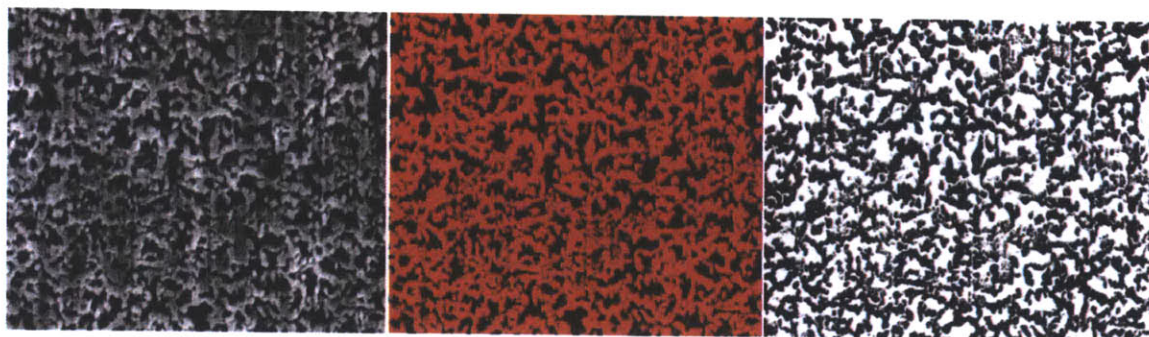
Figure 2.22. Grayscale to binary image conversion and analysis. The FIB cross-section is from a copper nanowire network on the Y21M clone. A) The original image contrast is maximized. B) The image is thresholded to identify the cross-section surface area. C) The image is converted to an 8-bit binary image for particle analysis. The nanowires are colored black. Image scale is 5.12 \mu m horizontal full width. This sample section has a determined porosity of 46.6%.
