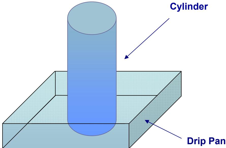
The cylinder broke and the fissile liquid collected in the drip pan. A blue flash was observed. The experimenter was splashed with liquid and, although he showered immediately, he later died.
