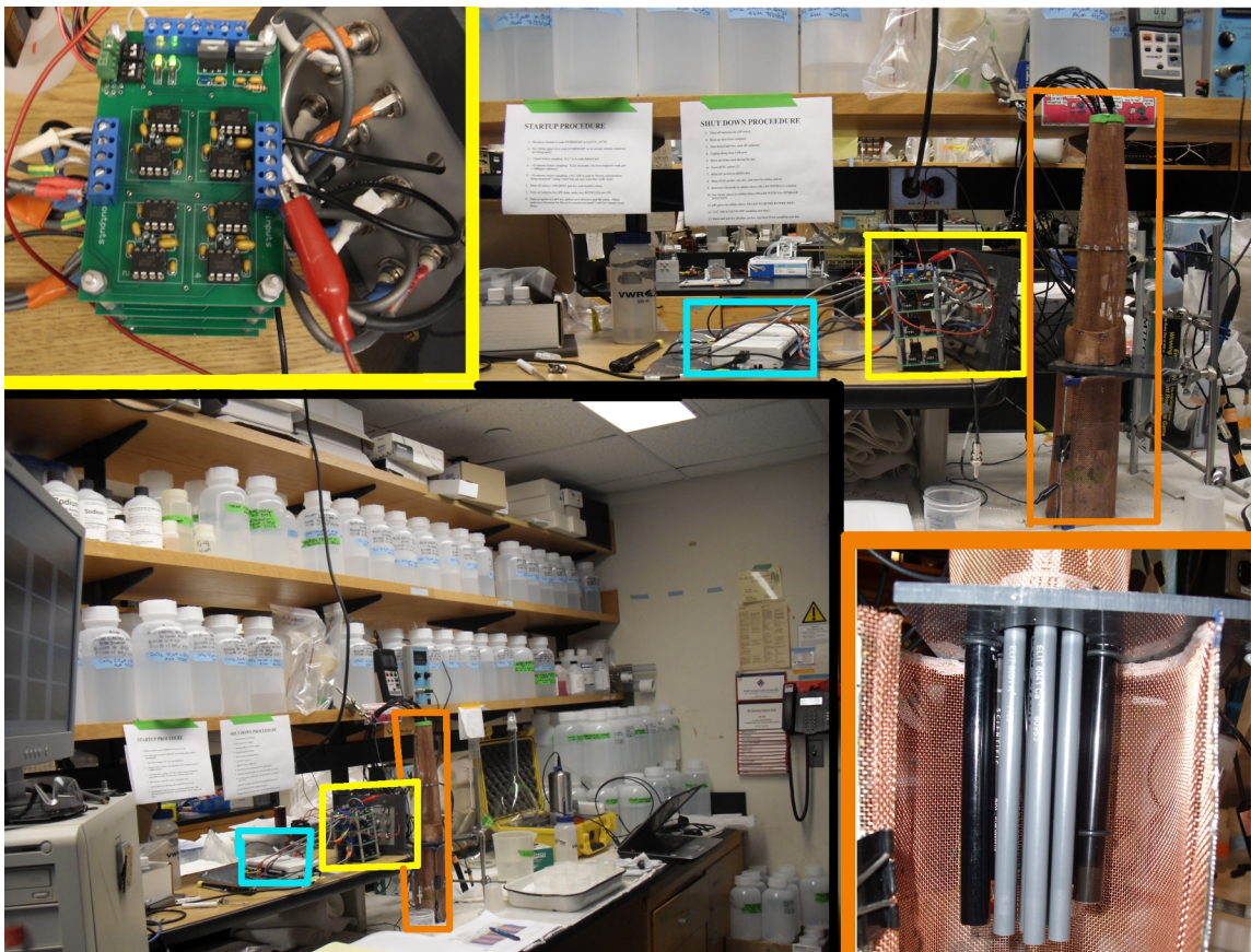
Figure 3-1: Photographs of lab setup for ISE sampling, including ISE hardware (orange), custom circuitry (yellow), data acquisition (teal), and PC for LabView interface (far left).
