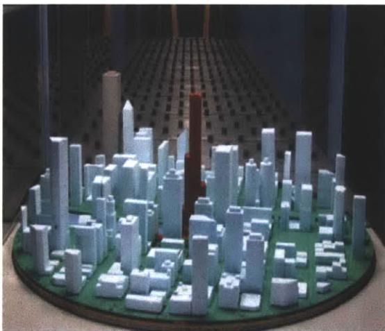
Figure 4: Chicago's Trump Tower in Wind Tunnel [5]
