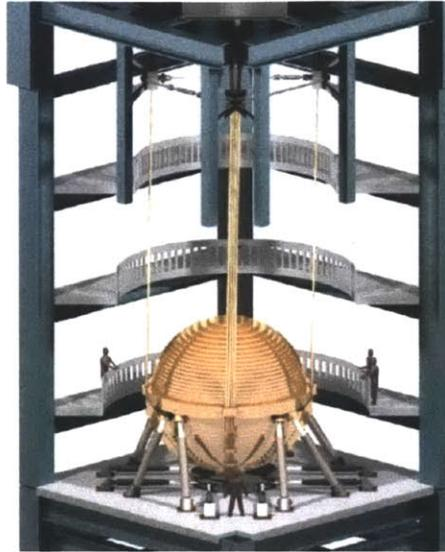
**Figure 15: Pendulum TMD in Taipei 101 [41]**
