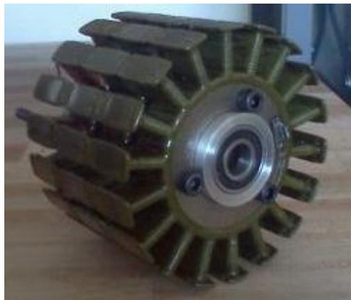
**Figure 3-4:** Picture of stator assembly.
