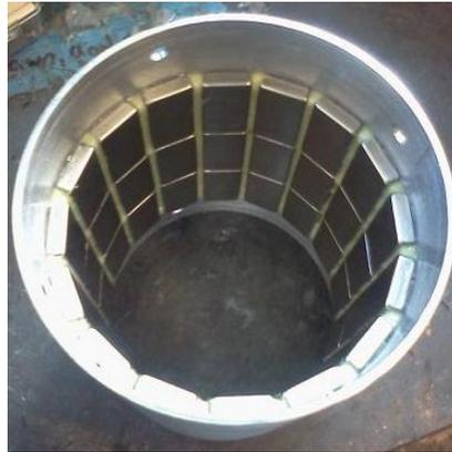
**Figure 3-5:** Picture of all the magnets in position with epoxy filling the gaps.
